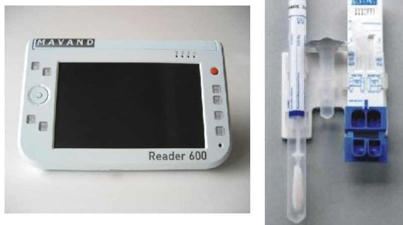
Figure 8. Rapid STAT mobile reader and test device: collection stick, buffer bottle and test panel.
