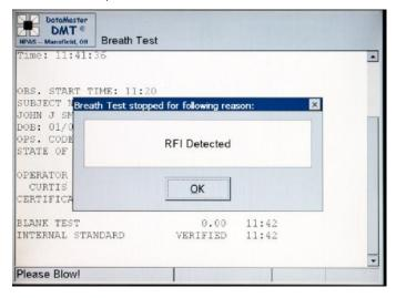
If the instrument gives an "RFI Detected" message on the display, touch the "OK" button, and the printout will also indicate "RFI Detected."
