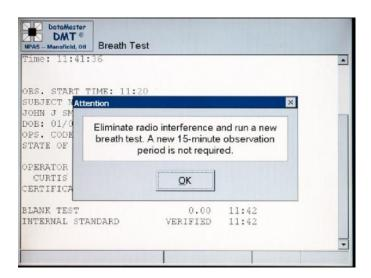
After the interference has been eliminated, touch the "RUN" button to initiate a new test. A new 15-minute observation **Error! Bookmark not defined** period is not necessary.
