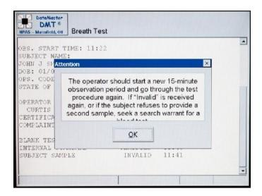
The operator should start a new 15-minute observation period and go through the test procedure again. If "Incomplete" is received again, or if the subject refuses to provide a second sample, seek a blood test. Diabetics, hemophiliacs and people with medical conditions requiring the use of an anticoagulant are unable to give consent to the withdrawal of their blood. Under those circumstances a search warrant will be required.
