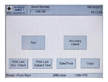
Step 2: Touch the "**DATE/TIME**" box in the bottom of the display.
