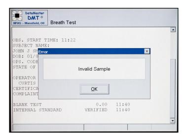
If, while the subject is blowing into the DATAMASTER DMT, he/she has a discontinuous breath flow, i.e. starts and stops blowing, or sucks back on the breath tube, the instrument may display "Invalid Sample."
