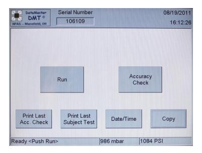
Step 1: Touch the "Accuracy Check" button, or hit the F5 button on the keyboard. This will bring up the "Operator Information" screen. The cursor will be in the "Last Name" box.
